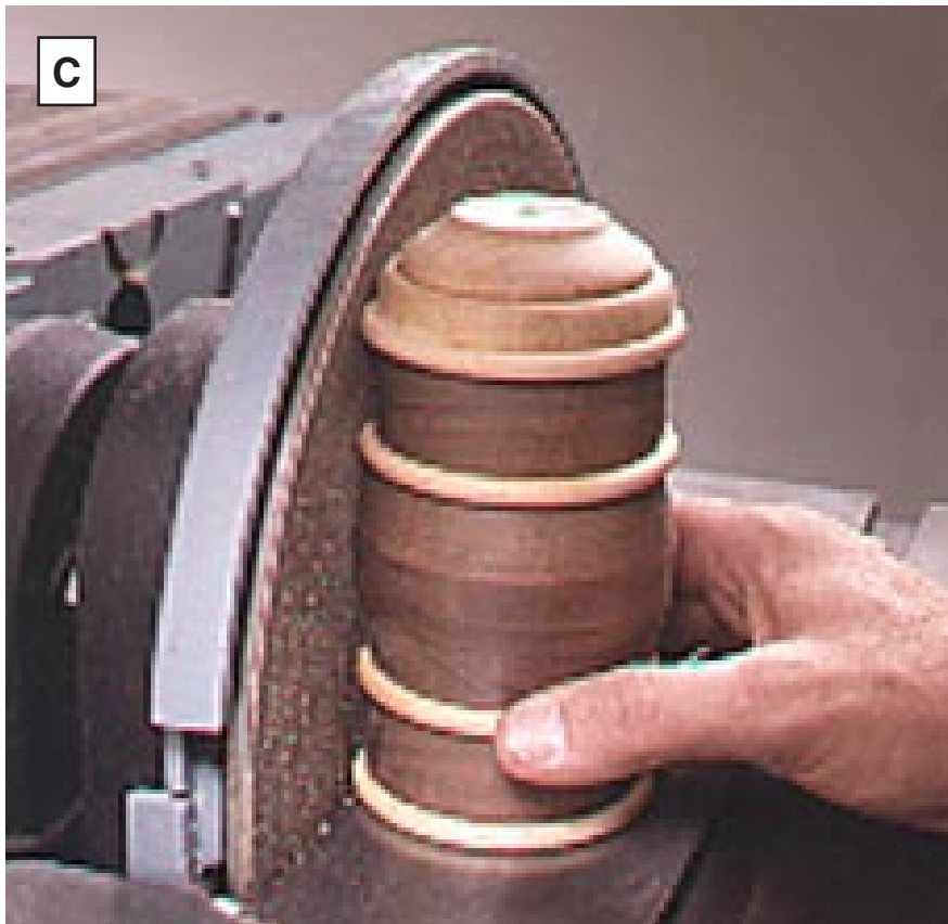
C Use a disc sander to sand a flat area on the bottom of the boiler for mounting the boiler to the chassis later.
