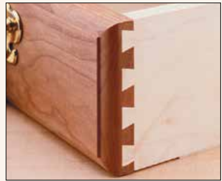
Half-blind dovetails are customary on a well-built drawer. I routed the joints using a hand-held router and dovetail jig.
