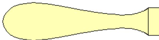
Diagram 8.4 Blending a bead and a cove to form a handle shape
