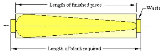
**Diagram 15.2: Allowing for the waste**
