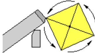
**Diagram 10.3 Position of roughing gouge at start of cut**
