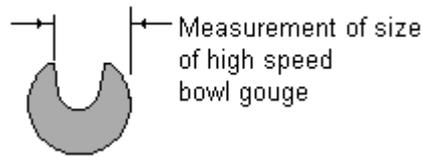
**Diagram 3.8 Measurement of size of HSS bowl gouge**
