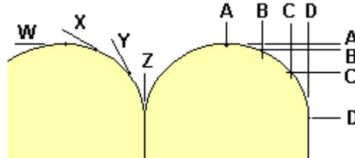
**Diagram 13.6** The stages in cutting a bead
