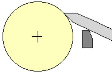
**Diagram 6.4 The bevel rubbing on an outside curve**
