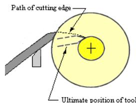
**Diagram 15.3: Maintaining the bevel in the rubbing position**
