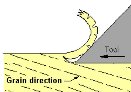
**Diagram 7.3 Cutting with the grain**
