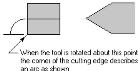
**Diagram 13.4 The arc described by the cutting point**
