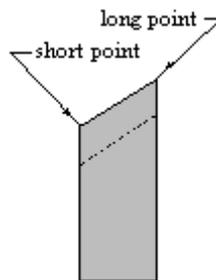
**Diagram 12.1 Naming the points of the skew chisel**
