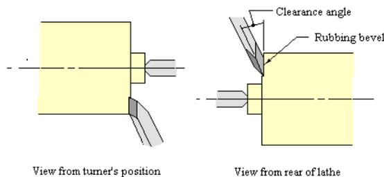
**Diagram 15.6: The rubbing bevel and the clearance angle.**
