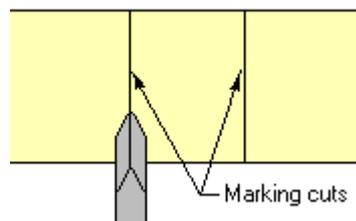
Diagram 14.1 The cuts made to mark the edges of a cove
