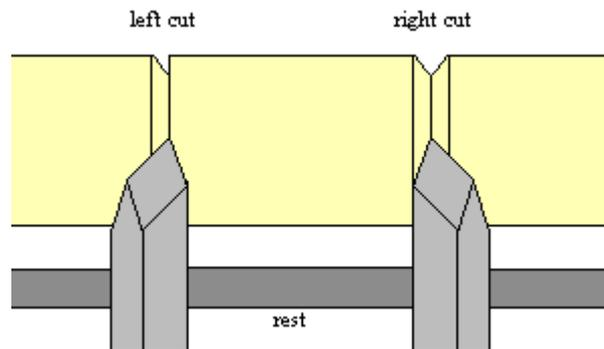
**Diagram 12.3 Leaning the chisel when making a cut**
