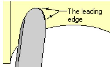
**Diagram 14.5 Cutting with the leading edge of the tool**
